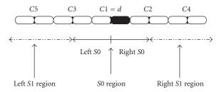
FIGURE 2: The 5 microcells model.
