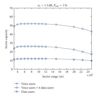
FIGURE 8: Sector capacity for different *R* for (voice users only, mixed services (voice users +5 data users), and data users only).
