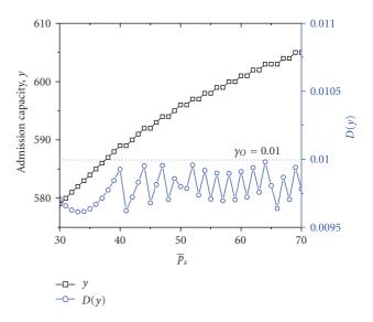
FIGURE 3: Relation between the admission capacity and the transmit power of the source node when transmitting its own traffic  $\gamma_O = 0.01$ ).
