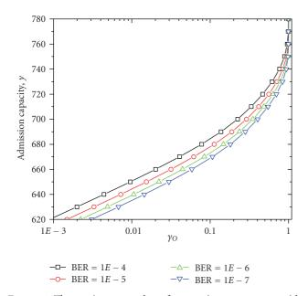
FIGURE 4: The maximum number of connections y versus  $y_0$  with respect to BER ( $\overline{p}_s = \overline{p}_r = 50 \text{ mW}, \sigma^2 = 10^{-11}, \phi = 100 \text{ Kbps}$ ).
