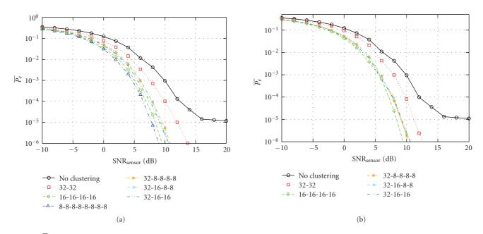
FIGURE 7:  $\overline{P}_e$  as a function of the sensor SNR, for different clustering configurations, ideal communication links, and the IEEE 802.15.4 MAC protocol. Case (a): absence of weighing; case (b): presence of weighing.
