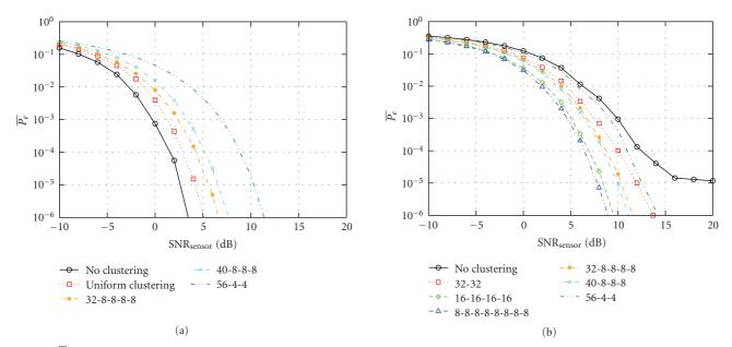
FIGURE 5:  $\overline{P}_e$  as a function of the sensor SNR, for different clustering configurations and ideal communication links. Case (a): ideal MAC; case (b): IEEE 802.15.4 MAC.
