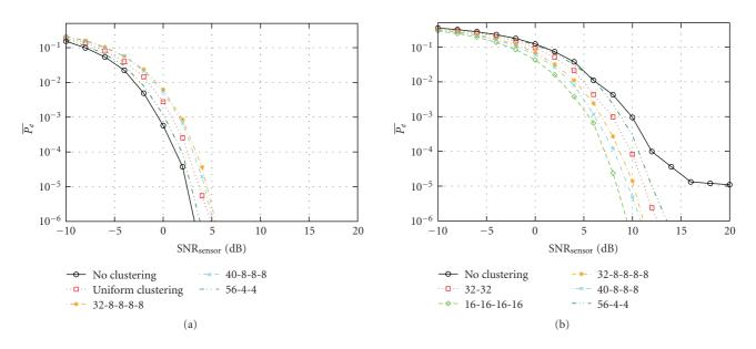
FIGURE 6:  $\overline{P}_e$  as a function of the sensor SNR, for different clustering configurations, ideal communication links, and weighing strategy at the AP. Case (a): ideal MAC; case (b): IEEE 802.15.4 MAC.
