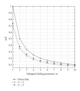
FIGURE 3: AoF for a dual-hop cooperative link with fixed gain relay and SC diversity receiver versus fading severity ( $m_1 = m_2 = m_0 = m$ ,  $\overline{\gamma}_1 = 1.5\overline{\gamma}_0$ ,  $\overline{\gamma}_2 = 3\overline{\gamma}_0$ , and  $\overline{\gamma}_0 = 0$  dB).
