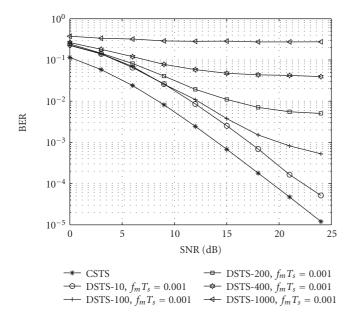
FIGURE 4: BER of DSTS (2 transmit antennas and 1 receive antenna) under Rayleigh fading channel with  $f_m T_s = 0.001$ , BPSK, DSTS with various segment sizes.
