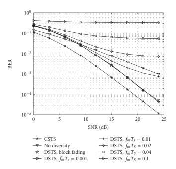
FIGURE 3: BER of DSTS (2 transmit antennas and 1 receive antenna) under block and Rayleigh fading channels with various  $f_m T_s$ , BPSK, DSTS with segment size of 10.
