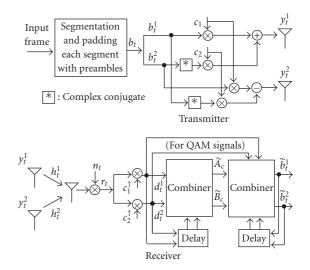
FIGURE 2: Transmitter and receiver of STS with differential detection.
