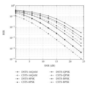
FIGURE 6: BER of DSTS (2 transmit antennas and 1 receive antenna) under Rayleigh fading channel with  $f_m T_s = 0.001$ , BPSK, QPSK, 8PSK, and 16QAM, DSTS with segment size of 10.
