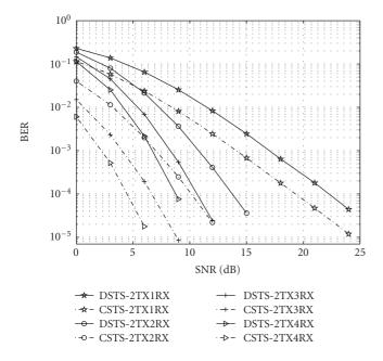
FIGURE 5: BER of CSTS and DSTS (2 transmit antennas and *N* receive antennas) under Rayleigh fading channel with  $f_m T_s = 0.001$ , BPSK, DSTS with segment size of 10.
