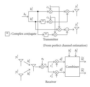
FIGURE 1: Transmitter and receiver of STS with coherent detection.
