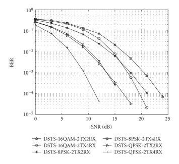
FIGURE 7: BER of DSTS (2 transmit antennas and N receive antennas) under Rayleigh fading channel with  $f_m T_s = 0.001$ , QPSK, 8PSK, and 16QAM, DSTS with segment size of 10.
