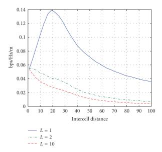
FIGURE 4: Spectral efficiency versus intercell distance (in meters) in the case of exponential path loss and multipath fading:  $\sigma^2 = 10^{-7}$ , P = 1,  $\gamma = 1$ , and L = 1, 2, 10.
