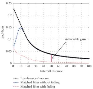
FIGURE 7: Spectral efficiency versus intercell distance (in meters) in the case of exponential path loss with fading, without fading, and
