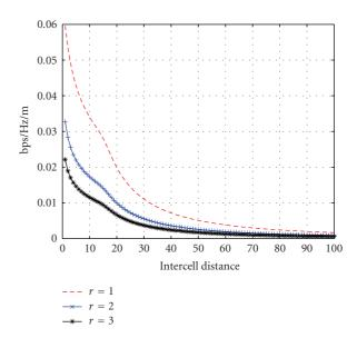
FIGURE 6: Effect of the reuse factor: spectral efficiency versus intercell distance (in meters) in the case of exponential path loss and fading:  $\sigma^2 = 10^{-7}$ ,  $\gamma = 2$ , P = 1, and r = 1, 2, 3.
