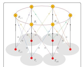
Figure 1 Uplink of C-GCMAC where N = 6 BSs are cooperating to decode all users' data; (the solid line illustrates intra-cell users and the dotted line shows inter-cell users). For simplicity, in this Figure there is only K = 1 user in each cell.
