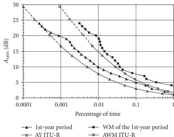
FIGURE 8: CDs of rain attenuation obtained for the first-year period.
