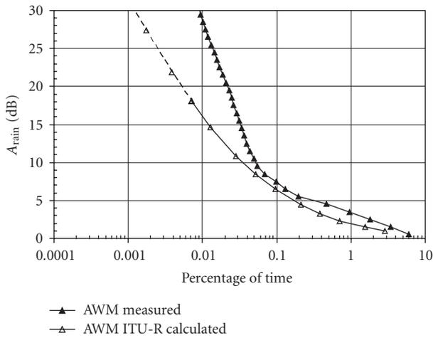
FIGURE 7: CDs of rain attenuation for AWM.
