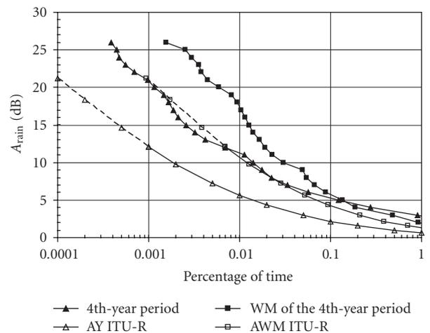
FIGURE 11: CDs of rain attenuation obtained for the fourth-year period.
