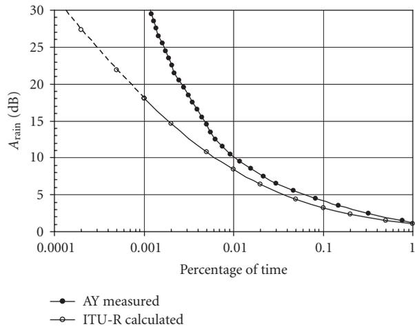
FIGURE 4: CDs of rain attenuation for AY.
