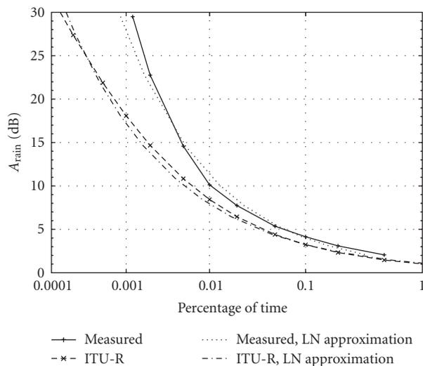
FIGURE 5: CDs of rain attenuation for AY and its LN approximations.
