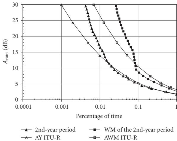
FIGURE 9: CDs of rain attenuation obtained for the second-year period.
