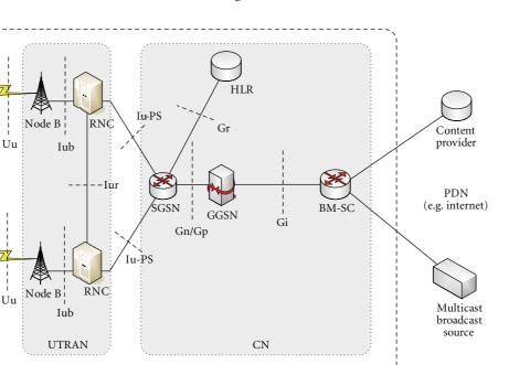
FIGURE 1: UMTS and MBMS architecture.
