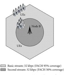
FIGURE 6: MBMS provision with rate splitting.
