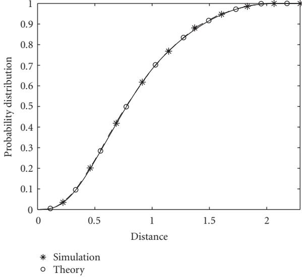
FIGURE 3: The distance probability distribution between nodes that are independent and uniformly distributed in a  $0.5 \times 1 \times 2$  cuboid space. The curve marked by “\*” is the result of simulation and that by “o” is the theoretical result.
