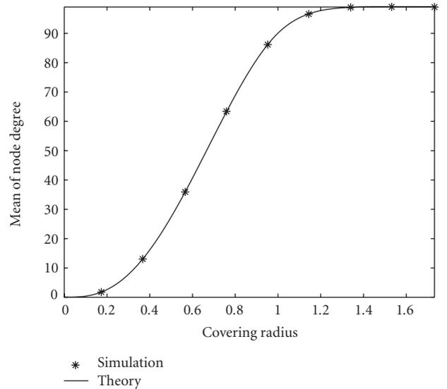
FIGURE 5: The average value of node degree of 100-node network in  $1 \times 1 \times 1$  cuboid space.
