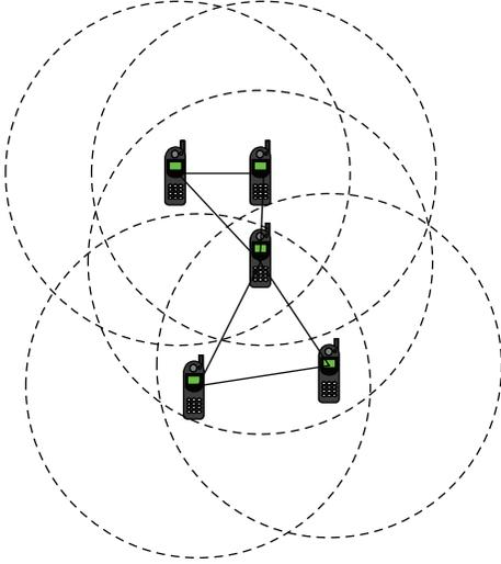
FIGURE 1: Random graph model of wireless ad hoc network.
