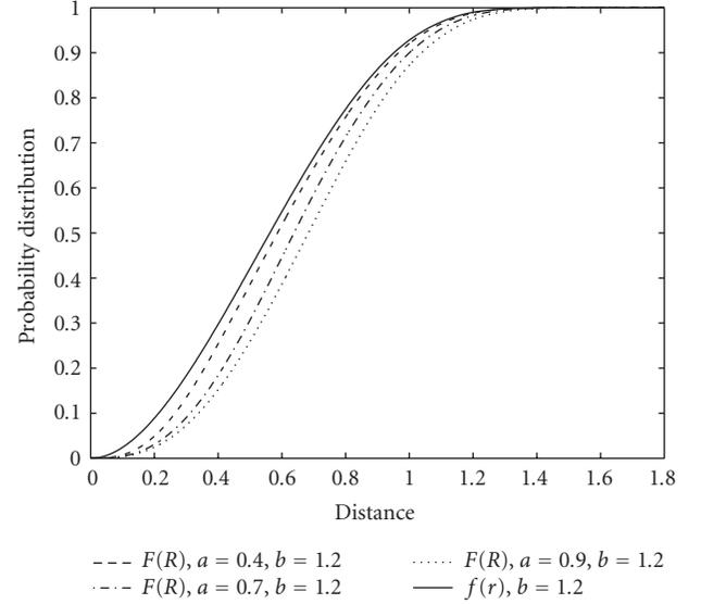
FIGURE 8: The comparison between  $f(r)$  and  $F(R)$  when  $a/b$  increases. The label “Distance” refers to  $R$  for  $F(R)$  and  $r$  for  $f(r)$ .
