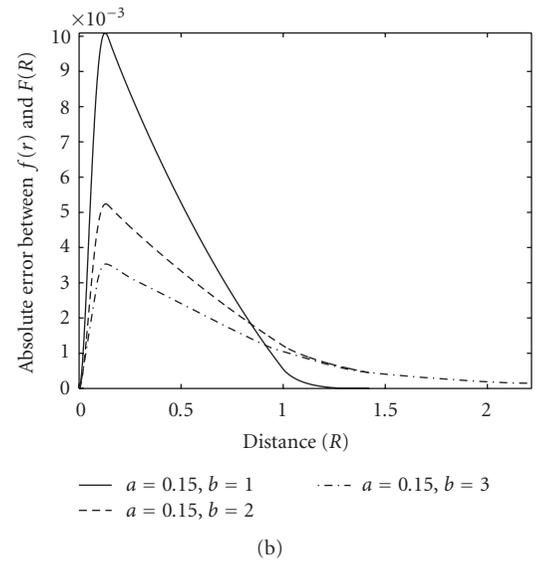
FIGURE 9: The relative error of using  $f(r)$  to estimate  $F(R)$  (a) for  $0.1 < R/a < 1.8$  and (b)  $1.8 < R/a < 5$ .
