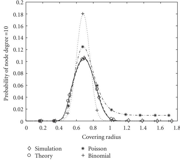
FIGURE 4: The probability of the node degree equals 10 in a 20-node network in  $1 \times 1 \times 1$  cuboid space.
