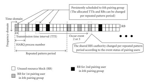
FIGURE 2: Resource assignment scenario with a resource sharing through user pairing.
