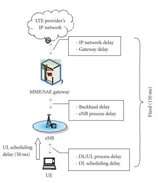
FIGURE 3: End-to-end delay components in E-UTRA.
