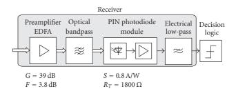
FIGURE 1: Setup of an optically preamplified receiver (*G*: preamplifier gain, *F*: preamplifier noise figure, *S*: photodiode responsivity,  $R_T$ : transimpedance).
