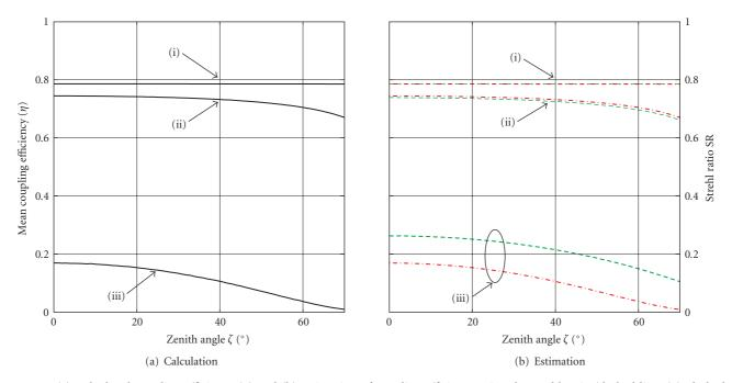
FIGURE 6: (a) Calculated coupling efficiency (1) and (b) estimation of coupling efficiency using the Strehl ratio (dashed line: (6), dasheddotted line: (7)) versus zenith angle for three different link scenarios: (i) GEO-to-HAP with  $h_{\text{HAP}} = 20 \text{ km}$  and D = 0.135 m, (ii) GEO-to-HAP with  $h_{\text{HAP}} = 2400 \text{ m}$  and D = 0.135 m, and (iii) GEO-to-ground with  $h_{\text{ground}} = 2400 \text{ m}$  and D = 1 m at the OGS.
