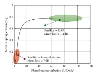
FIGURE 5: Mean coupling efficiency  $\langle \eta \rangle$  for a standard single-mode fiber as a function of the rms phasefront perturbation RMS<sub> $\lambda$ </sub> given in fractions of the wavelength  $\lambda$ .
