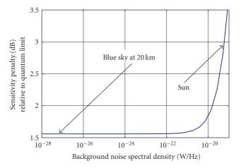
FIGURE 2: Calculated receiver sensitivity penalty of an optically preamplified receiver using RZ intensity modulation at a bit error probability of  $10^{-9}$  as a function of background noise power spectral density.
