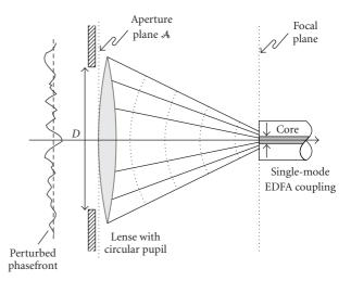
FIGURE 4: Coupling geometry: A thin lens focuses the incident field *E*, which is assumed to have constant amplitude but a statistically disturbed phase, onto the bare end of a single-mode fiber.
