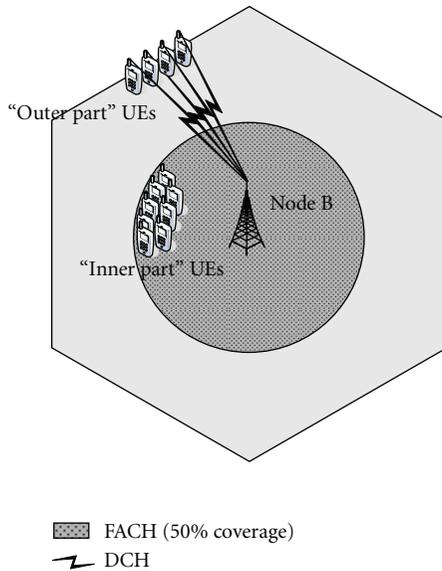
FIGURE 7: . MBMS provision with Mixed DCHs and FACH.
