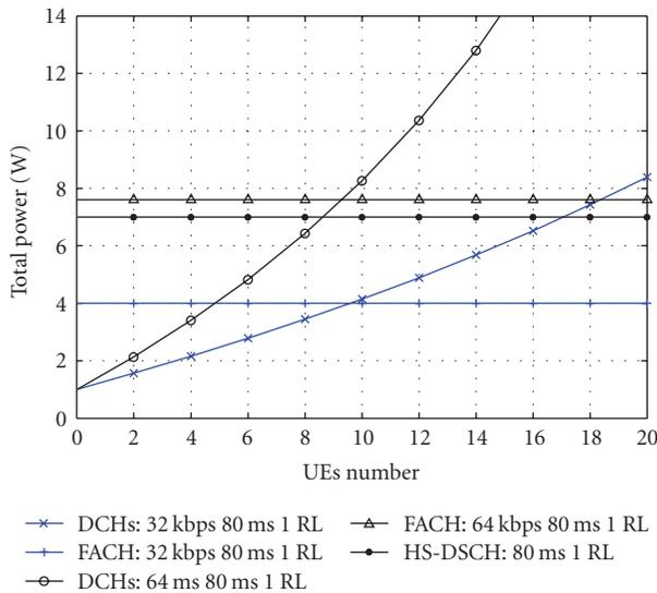
FIGURE 10: Node B's Tx power for 95% coverage.
