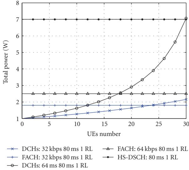
FIGURE 9: Node B's Tx power for 50% coverage.
