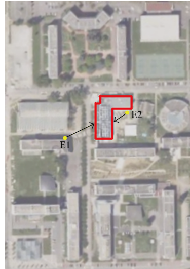
FIGURE 2: Outdoor to indoor scenario. In red: the building where the indoor measurements were performed. E1 and E2 represent the position of each emitter and the black arrows show the directions where the directive antennas were pointing.
