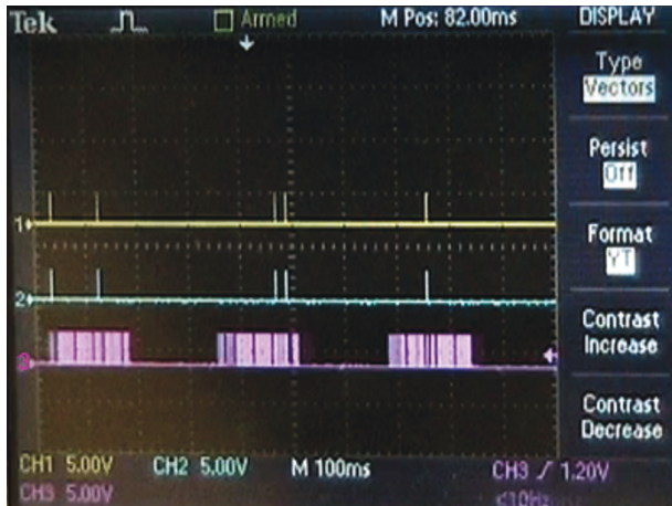
FIGURE 22: Implementation of WisperNet-Time showing changing patterns on a frame-by-frame basis.
