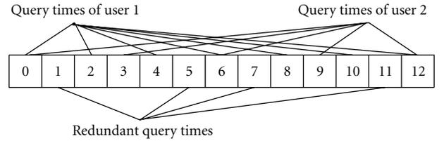
FIGURE 2: Example of multirate query.
