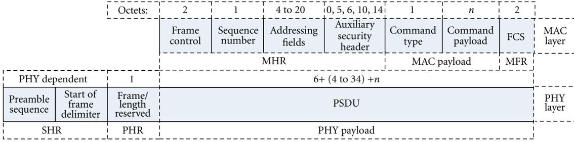
FIGURE 5: MAC command frame and the PHY packet.
