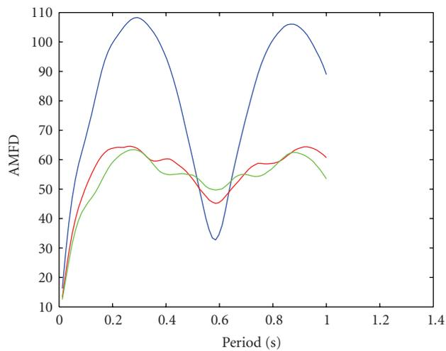
FIGURE 16: AMDF of accelerometer data during walking.
