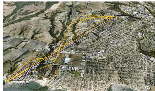
FIGURE 18: GPS data from the test deployment. The yellow track was logged by the GPS on a CSN carried by a researcher. The black track is the GPS data from the CSN carried by a domestic dog. An SRN was located at Long Marine Lab, Santa Cruz, CA, USA (A). The dog lived at B and his owner worked at A. Data was successfully transferred to the SRN via hops 1 and 2.
