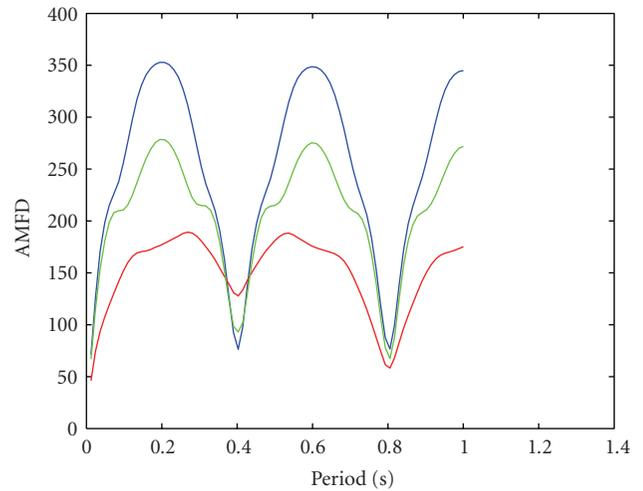
FIGURE 17: AMDF of accelerometer data during running.
