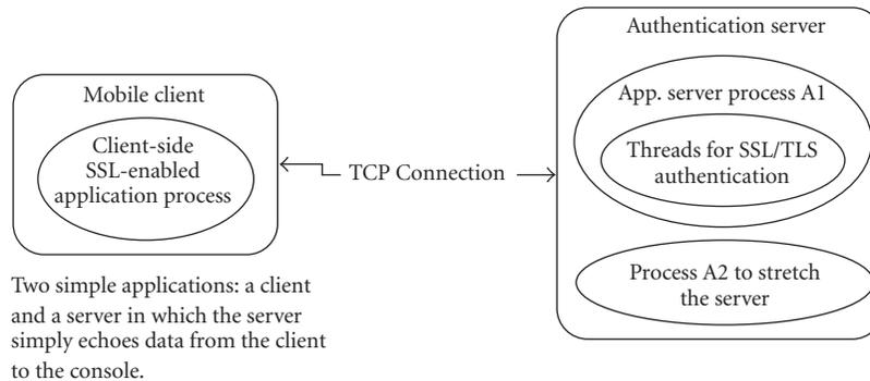
FIGURE 8: Software architecture.
