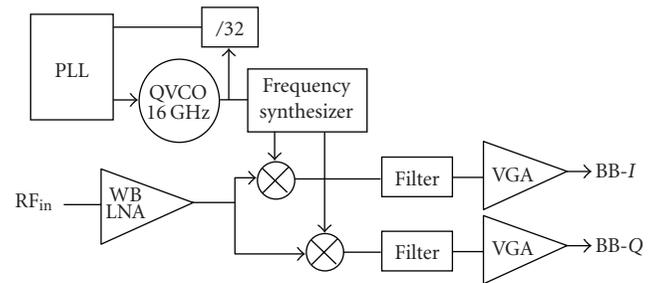
FIGURE 9: Receiver architecture used in [13]. The PLL is implemented off-chip.
