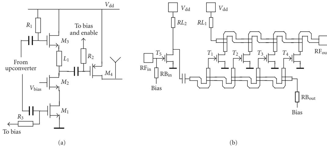
FIGURE 5: Two implementations of a CMOS RF PA: an inductively loaded PA (a), and a distributed PA (b).
