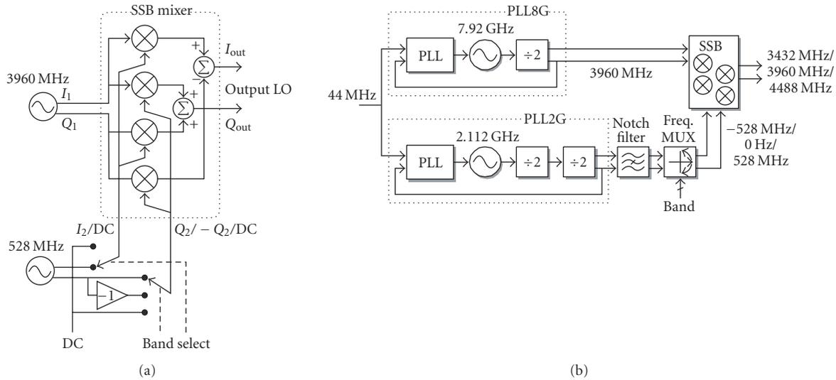
FIGURE 6: LO scheme based on SSB mixing (a) and a possible implementation (b).
