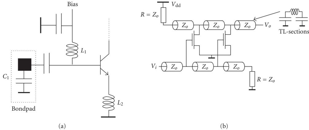
FIGURE 3: Several LNA topologies: wideband impedance matching (a); distributed LNA (b).
