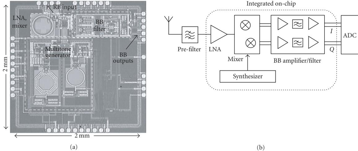
FIGURE 10: Chip photograph (a) and block diagram (b) of a fully integrated UWB receiver.
