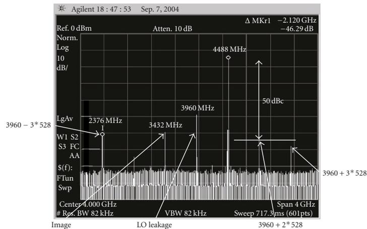
FIGURE 7: Measured spectral output of the synthesizer in [16] when generating the LO for band #3.
