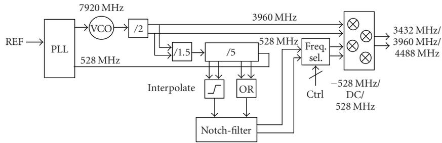
FIGURE 8: Single PLL, single SSB mixer synthesizer implementation.
