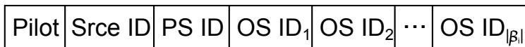
Figure 2 Report packet structure. Pilot is used to estimate channel state from a sender in D to a receiver in R . SrceID is the source identification, PSID is the current sink node identification, and OSID i is the destination node identification of the i th stored packet in the buffer of the current sink node. \beta_i is the set of the packets overheard by the current node d_i .
