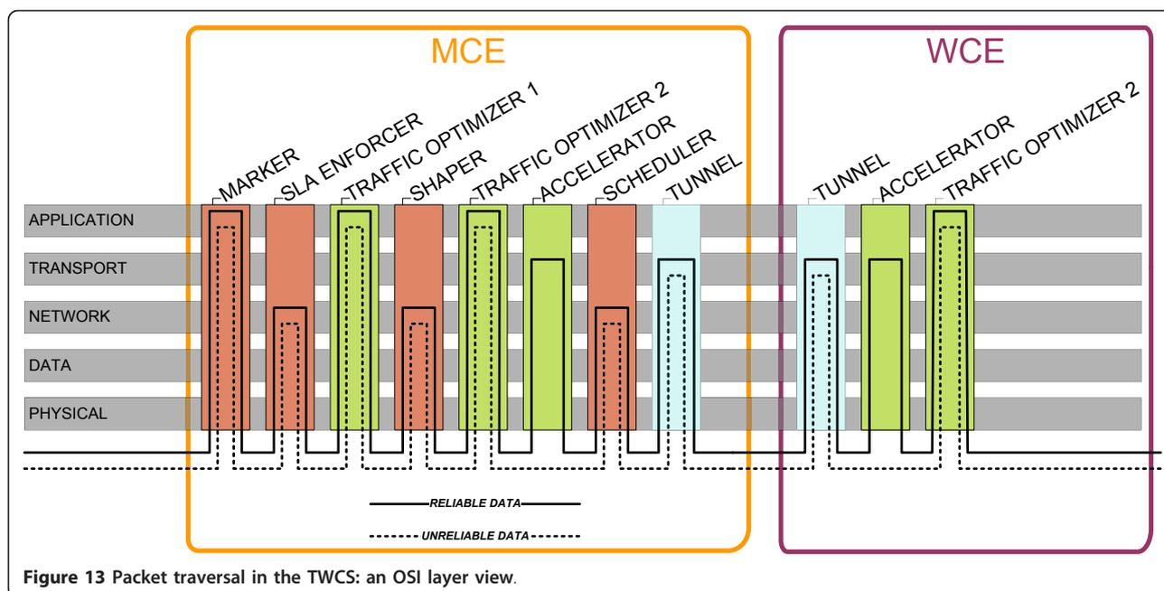
**Figure 13** Packet traversal in the TWCS: an OSI layer view.
