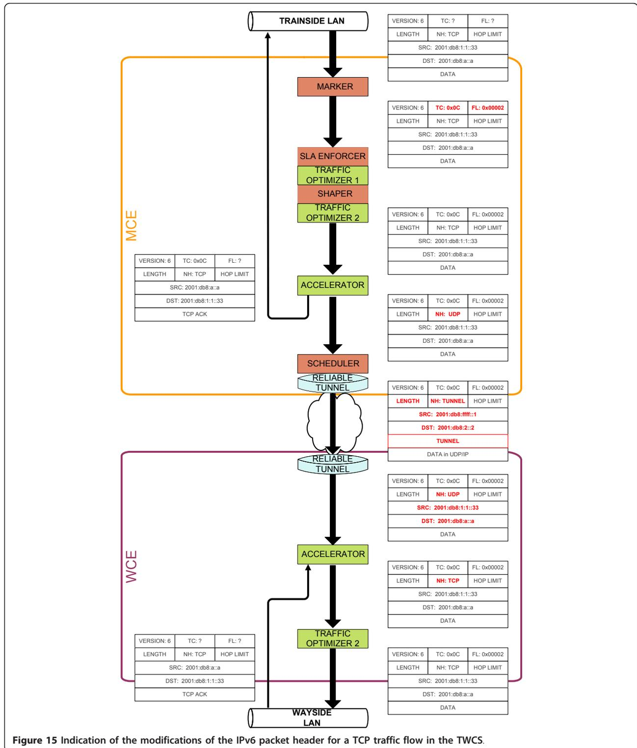
Figure 1). TCP ACKs that are received as a reply to this packet, will be discarded by the Accelerator at the WCE, as the packet was already acknowledged by the transmitting Accelerator at the MCE.
