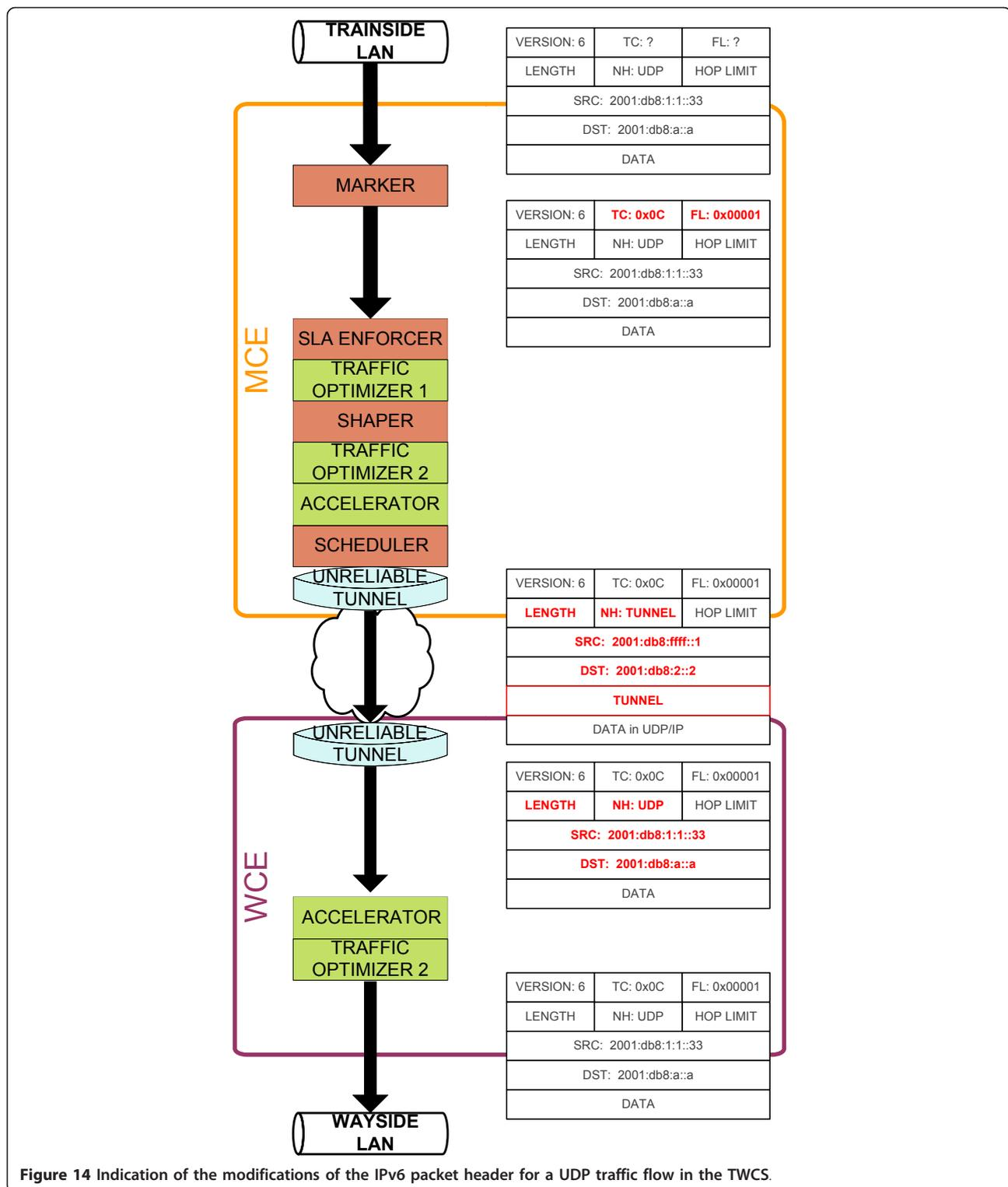
flows. The source IP address of the new packet is the IP address of the wireless interface, which is here assumed 2001:db8:fff::1 (see Figure 9) and the destination address is the IP address of the WCE, which is here assumed 2001:db8:2::2 (see Figure 9).
