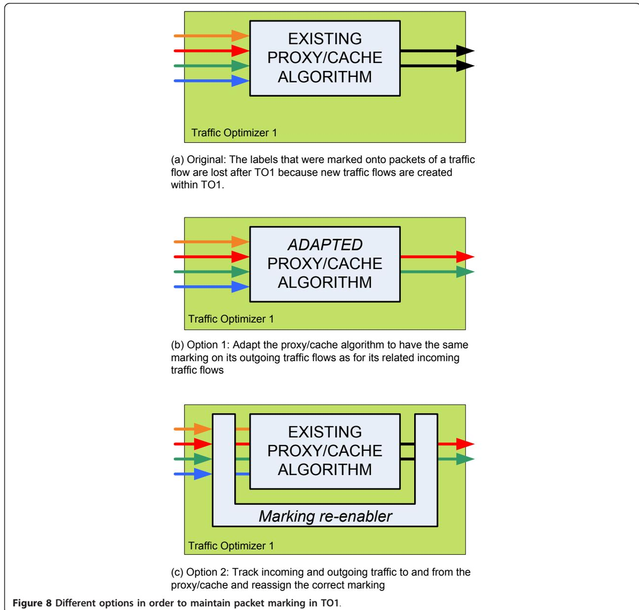
marking to each outgoing traffic flow, as shown in Figure 8c. However, it would nevertheless be a difficult task to match the correct incoming traffic flow to the outgoing one.
