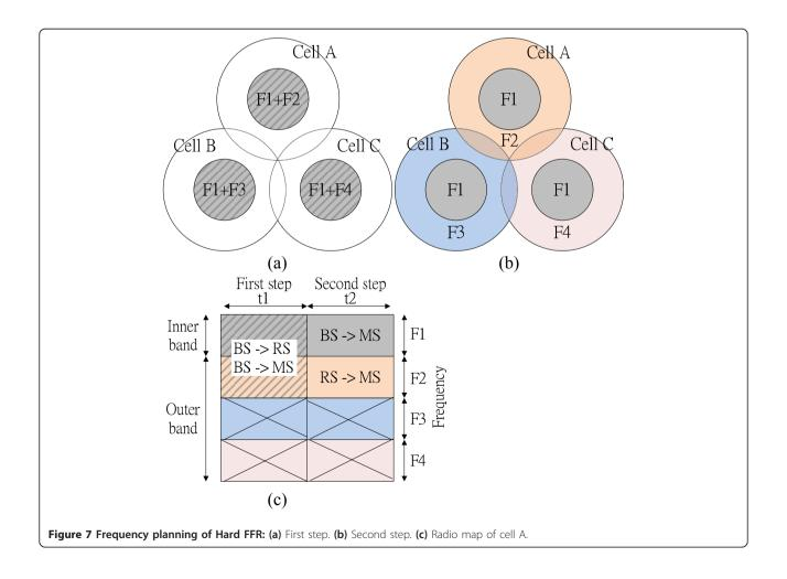
users at the same time, as shown in Figure 7b. In cell A, outer users receive data from RSs through the outer band (F2) with no interference. Although the BSs in cells B and C cause interference on the inner band, inner users in cell A who have a good SINR can still receive data successfully. The radio map of cell A is shown in Figure 7c.
