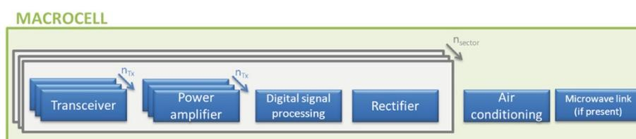
Figure 1 The architecture of a macrocell base station.
