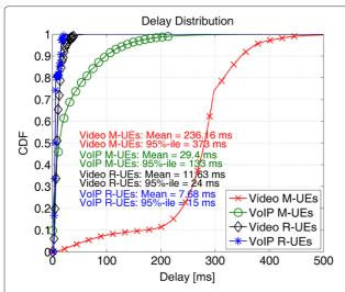
Figure 14 DeNB+2RN scenario with conventional resource allocation (Fair-RU resource partitioning plus proportional fair scheduler): delay CDF comparisons for different UE groups (M-UEs and R-UEs) and traffic types (VoIP and video).
