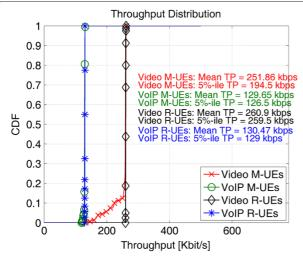
Figure 11 DeNB+2RN scenario with proposed QoS-aware resource allocation: throughput CDF comparisons for different UE groups (M-UEs and R-UEs) and traffic types (VoIP and video).
