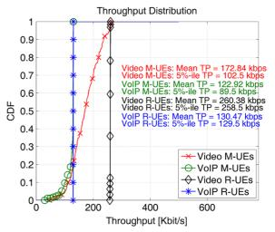
Figure 13 DeNB+2RN scenario with conventional resource allocation (Fair-RU resource partitioning plus proportional fair scheduler): throughput CDF comparisons for different UE groups (M-UEs and R-UEs) and traffic types (VoIP and video).
