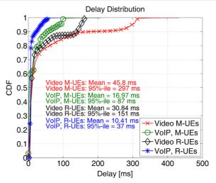
Figure 12 DeNB+2RN scenario with proposed QoS-aware resource allocation: delay CDF comparisons for different UE groups (M-UEs and R-UEs) and traffic types (VoIP and Video).
