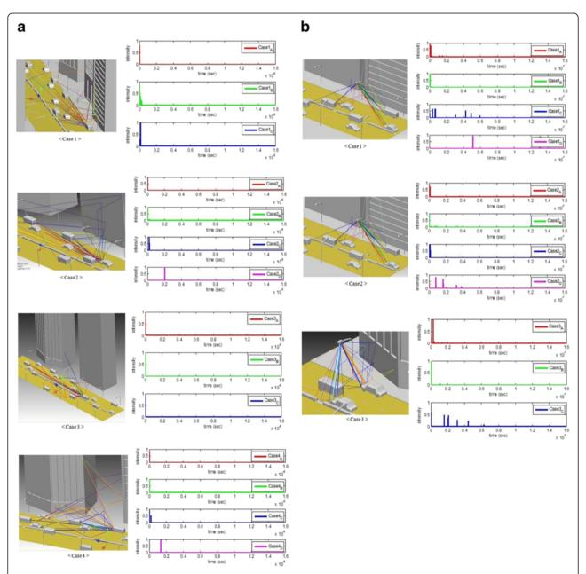
Figure 9 The VLC channel impulse responses in the metropolitan street scenario: (a) the four scenes for the V2V communication and corresponding channel impulses; (b) the three scenes for the V2V communication and corresponding channel impulses.
