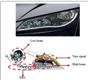
Figure 1 The LED headlamp structure (refence model: Audi R8 headlamp).
