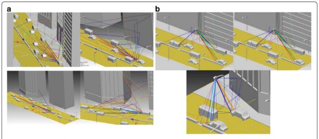
Figure 7 The VLC scenes for the V2V and V2I communication link in metropolitan street scenario: (a) the four scenes for the V2V communication link; (b) the three scenes for the V2I communication link.
