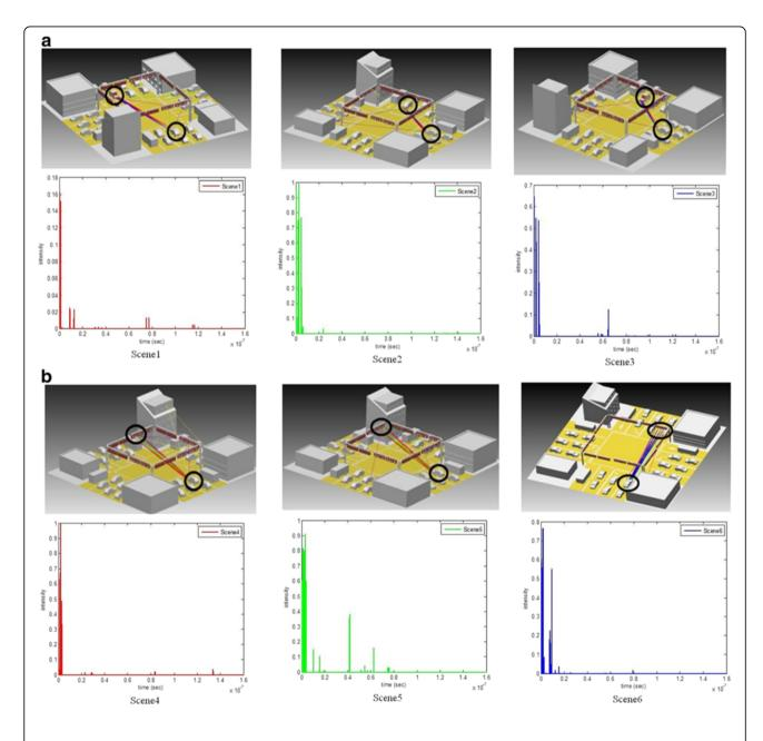
Figure 8 The VLC channel impulse responses in the crossroad scenario: (a) the three scenes for the V2V communication and corresponding channel impulse responses; (b) the three scenes for the V2I communication and corresponding channel impulse responses.
