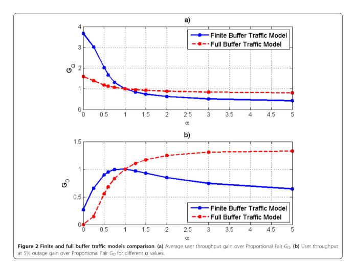
Hence, the results show that the relative comparison of KPIs, such as the average user throughput or the user throughput at 5% outage, between two different  $\alpha$  values of the  $\alpha$ -fair gradient scheduling algorithm, is insensitive to the network load under the full buffer traffic model. However, the same relative comparison is indeed load sensitive under the finite buffer traffic model.
