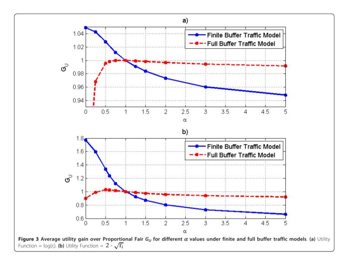
performance of  $\alpha = 0.6$  and  $\alpha = 1$ . For finite buffer, the offered load *L* = 11 Mbps is used.
