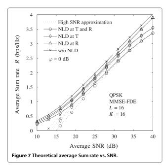
terminal (i.e., transmitter and relay) is nonlinear HPA present. We observe that the average sum-rate performance is more sensitive to the nonlinear HPA introduced at source. This is because the signal affected by the nonlinear HPA is transmitted in the second stage as well (over the relay), and consequently, the worse performance is obtained. We note here that the average sum-rate upper bound also performs well in the low SNR region.
