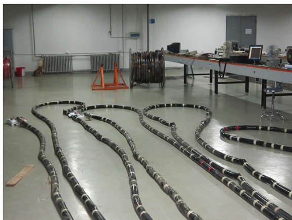
Figure 1 Actual hydrophone line array debugged in processing workshop. Hydrophones were distributed uniformly on the tow rope laid on the ground. The PC in the upper right corner of the figure is mainly used to store real-time data and reflected echo.
