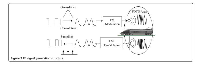
be realized by a pre-modulation low-pass filter (a general Gaussian low pass filter (LPF)) and a frequency modulation (FM) modulator. The Gaussian low pass filter can be represented by:
