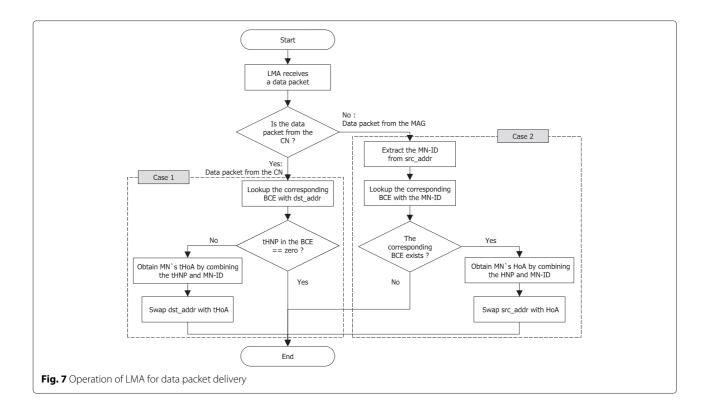
(2) If there is no BCE corresponding to the MN-ID, the LMA does not swap the src\_addr with the HoA and sends the data packet to the CN. Otherwise, the LMA swaps the src\_addr in the IP header of the data packet with the HoA and sends the data packet to the CN. The MN's HoA is obtained by combining the HNP and the MN-ID.
