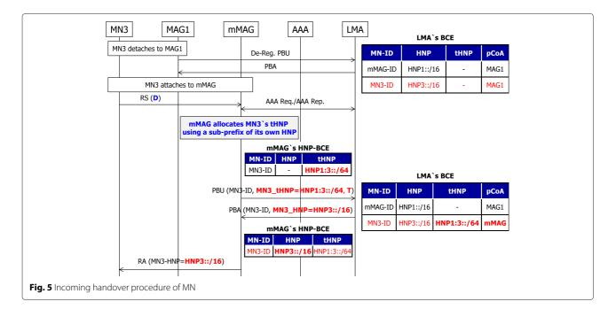
mMAG and LMA have an IP address swapping function that changes either the source address or the destination address in the IP header of the data packet to a tHoA or the HoA.
