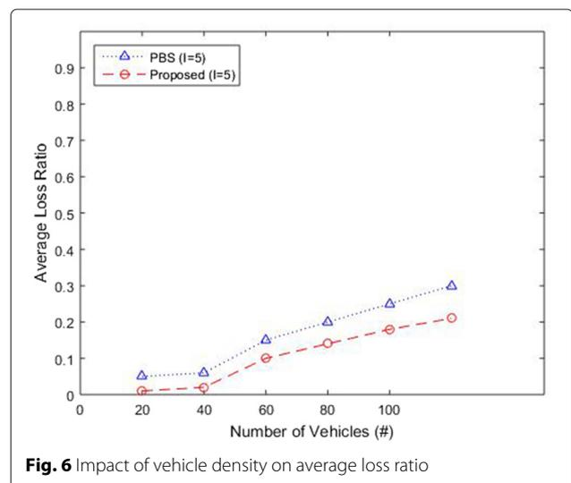
**Fig. 6** Impact of vehicle density on average loss ratio
