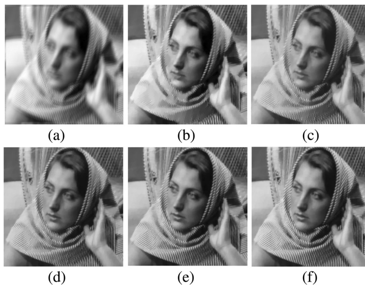
Fig. 5 Experiments on the blurred image “Barbara” (degrade by a 19 \times 19 kernel). a Blurred image (PSNR = 18.17). b The local TV [5] (PSNR = 20.12, t = 6.36 s). c GOS_TV [15] (PSNR = 21.38, t = 8.85 s). d The local/nonlocal TV [26] (PSNR = 22.89, t = 26.77 s). e The nonlocal TV [8] (PSNR = 23.34, t = 14.32 s). f The proposed model (PSNR = 24.93, t = 13.03 s)
