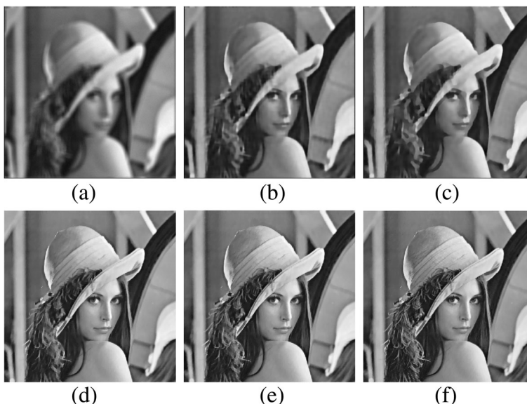
Fig. 7 Experiments on the blurry and noisy image of “Lena” ( 512 \times 512 ). a Blurry and noisy (PSNR = 19.31). b The local TV [5] (PSNR = 21.22, t = 4.32 s). c GOS_TV [15] (PSNR = 23.09, t = 10.93 s). d The local/nonlocal TV [26] (PSNR = 24.57, t = 20.21 s). e The nonlocal TV [8] (PSNR = 25.69, t = 14.34 s). f The proposed model(PSNR = 27.53, t = 13.02 s)
