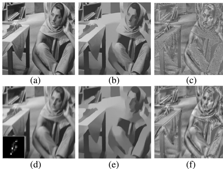
Fig. 1 Image regions division. a Original image. b Edges and constant regions of (a). c Details of (a). d Blurred image(PSNR = 19.24). e Edges and constant regions of (d). f Details of (d)
