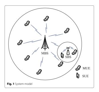
The first slot is for MUE data communication with time  $\tau_0$ . It is assumed that the SUEs can harvest energy from the received signals transmitted by the MUEs in this slot. The second slot with time  $\tau_1$  is for the SBS to broadcast energy wirelessly to the SUEs with transmit power  $p_{\rm SBS}^s$ . The third slot with time  $\tau_2$  is for the SUEs to use harvested energy from the former two slots to transmit data to the SBS.
