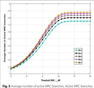
Fig. 5 Average number of active MRC branches. Active MRC branches versus output SNR for different numbers of antennas M with  $M_c = 2$  and  $\Psi_1 = 10 \text{ dB}$
