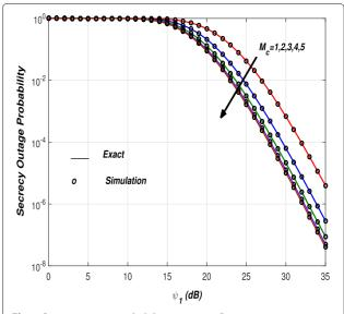
**Fig. 2** Secrecy outage probability versus  $\psi_1$ . Secrecy outage probability versus SNR of the main channel  $\psi_1$  for different numbers of selected antennas  $M_c$  with  $R_s = 1$ ,  $\Psi_2 = 10$  dB,  $\Psi_t = 10$  dB,  $\sigma = 1$ , and M = 7
