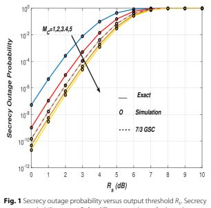
outage probability versus  $R_s$  for different numbers of selected antennas  $M_c$  with  $\psi_1 = 30$  dB,  $\Psi_2 = 10$  dB,  $\Psi_t = 7$  dB,  $\sigma = 0.5$ , and M = 7. Solid line represents the exact result and block dots represent the simulation result
