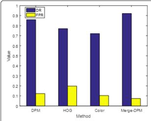
**Fig. 6** Comparison of different vehicle target detection algorithms. DR vehicle detection rate, FPR vehicle false positive rate
