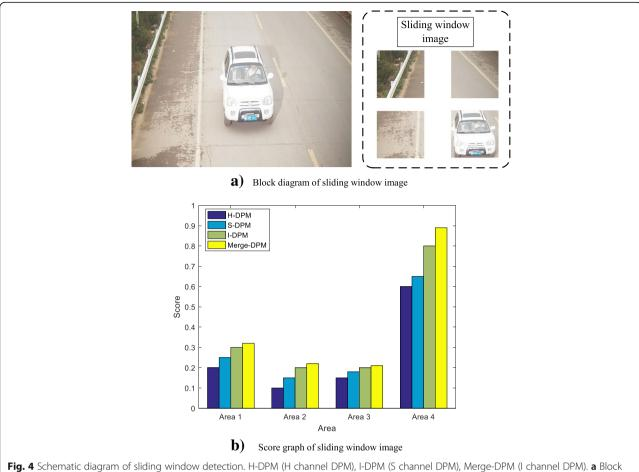
Fig. 4 Schematic diagram of sliding window detection. H-DPM (H channel DPM), I-DPM (S channel DPM), Merge-DPM (I channel DPM). a Block diagram of sliding window image. b Score graph of sliding window image
