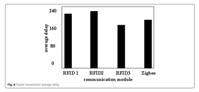
time of module based on ZigBee technology is the second, which concentrating between 170 ms and 193 ms, and the average transmission delay is 186.89 ms. By the analysis of the above test results, the communication models based on ZigBee technology, the single transmission volume of uplink and downlink data packets is the largest, and the transmission delay is moderate to be recommended for building wireless sensor networks.
