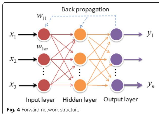
Fig. 4 Forward network structure
