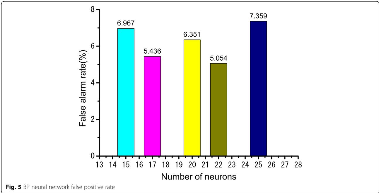
**Fig. 5** BP neural network false positive rate
