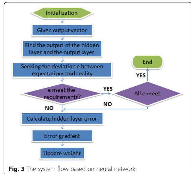
Fig. 3 The system flow based on neural network
