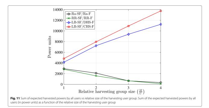
the optimum value of the objective function. Additionally, as more users are able to recharge their batteries (see Fig. 11), they can decode higher rates in future frames. Nonetheless, from a given size  $\frac{M}{U}$  on, the system sum rate starts to decrease as the harvesting constraints become active, although the problem is always feasible, and users recharge their batteries, as is indirectly depicted in Fig. 11.
