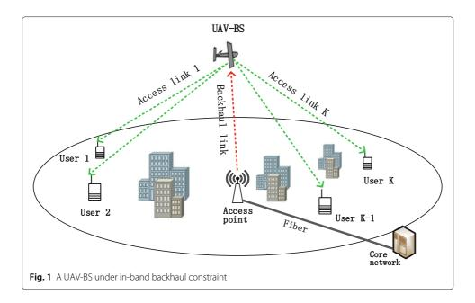
link between the AP and the UAV-BS as backhaul link and that between the UAV-BS and user *k* as access link  $k, \forall k \in \mathcal{K}$ . We consider the downlink communication from the UAV-BS to the users, and our work can be extended to the uplink communication scenario straightforwardly.
