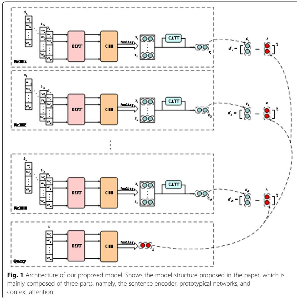
**Fig. 1** Architecture of our proposed model. Shows the model structure proposed in the paper, which is mainly composed of three parts, namely, the sentence encoder, prototypical networks, and context attention
