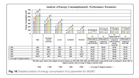
destination, and later these relay nodes are prioritized. Finally, the performance of the proposed WGWO protocol is compared with the existing ETSSEP, LCM, partition-based LEACH, and TBC, respectively, in terms of delay, energy consumption, network lifetime, throughput, and delivery ratio. The results attest that the efficiency of the hybrid WGWO based clustering scheme is much better than the various existing schemes.
