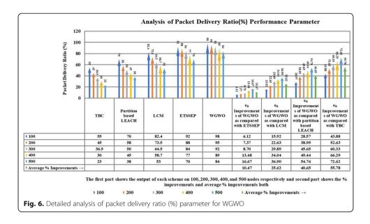
300, 400, and 500 nodes, and later in this figure, these five different columns represent the percentage improvements, and finally, sixth columns represent average percentage improvements comparing with each scheme, respectively.
