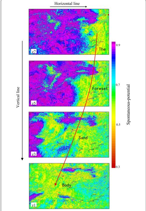
**Fig. 6** Horizon slice of the intermediate section in Member 3 of the Shahejie Formation in the Dongying Delta as obtained by multi-attribute SP inversion. The yellow is sand, green is silt, purple is mud, and blue is silty-mud.
