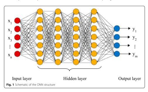
the output layer are determined by the weights [11, 12]. In this study, a DNN consisting of one input layer, one output layer, and three hidden layers was used. Herein, a convolution operator is involved, and the seismic attribute is convoluted with the convolution operator before being used as the input of the DNN.
