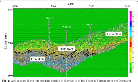
**Fig. 5** Well section of the intermediate section in Member 3 of the Shahejie Formation in the Dongying Delta as obtained by multi-attribute SP inversion
