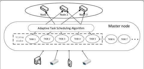
**Fig. 3** Task scheduling schematic. How the adaptive task scheduling algorithm optimally schedules tasks on edge nodes
