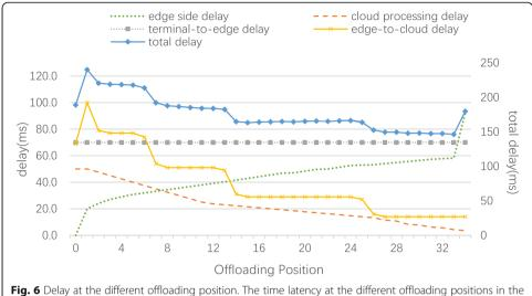
**Fig. 6** Delay at the different offloading position. The time latency at the different offloading positions in the ResNET-34 Model
