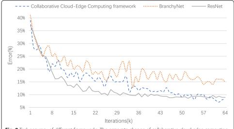
**Fig. 9** Task accuracy of different frameworks. The error rate change of collaborative cloud-edge computing, BranchyNet, and ResNet framework as the number of iterations increases
