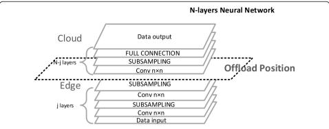
**Fig. 2** Cloud-edge offloading schematic. The neural network architecture that is divided into two parts for deployment at the edge and the cloud as an example
