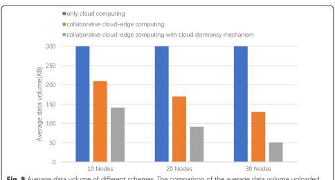
**Fig. 8** Average data volume of different schemes. The comparison of the average data volume uploaded from only cloud computing scheme, collaborative cloud-edge computing scheme, and the scheme with cloud dormancy mechanism
