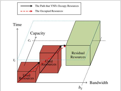
**Fig. 3** The bin. This is the bin which each MEC server is regarded. In this architecture, we denote its storage, virtual link bandwidth requirements, and usage time as a three-dimensional vector of capacity-bandwidth-time
