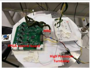
Fig. 4 The hardware experimental circuit and the WA mode of the HRG
