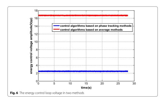
energy control voltages are recorded by upper-computer software, as shown in Fig. 6. Obviously, the phase tracking method in the paper, the energy control voltages could decrease an order of magnitude. It means that the energy transition efficiency increases by an order of magnitude.
