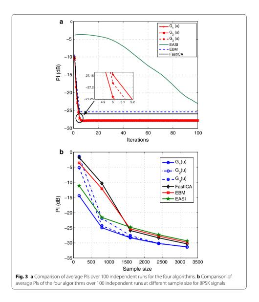
addition, it can also be seen that the convergence speed and convergence values of the proposed algorithm using the three different function G(u) are similar, and the convergence values of the proposed algorithm are lower than the two comparing algorithms.
