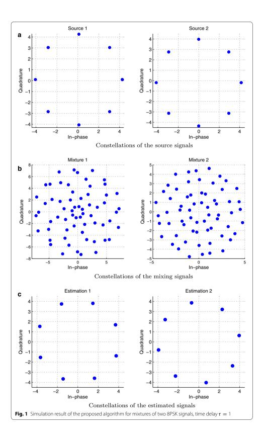
$\lambda = 0.3$ . In this simulation, the two 8PSK are with the following parameters: symbol rate  $R_s = 198$  kBps and raised cosine filter which has 0.35 roll-off factor, sampling frequency is  $16R_s$ . The mixing matrix is randomly generated as
