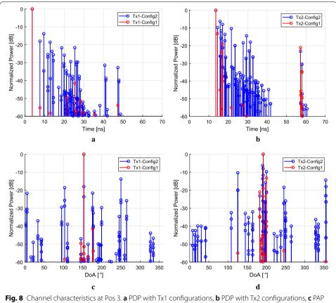
with Tx1 configurations and d PAP with Tx2 configurations
