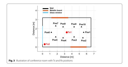
around the table with their wireless equipment at 1 m height are highlighted with triangles in Fig. 3.
