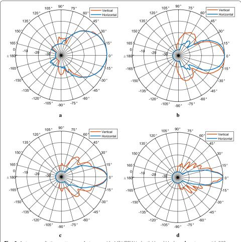
**Fig. 6** Antenna radiation patterns. **a** Antenna with 44° HPBW in both V and H-plane, **b** antenna with 29° HPBW in both V and H-plane, **c** antenna with 16.5° HPBW in both V and H-plane and **d** antenna with 10° HPBW in both V and H-plane
