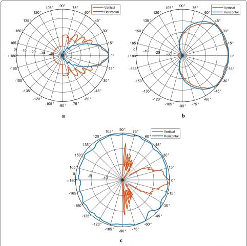
**Fig. 2** Antenna radiation patterns, **a** Antenna with 10° and 13° HPBW in V and H-plane, respectively, **b** antenna with 100° HPBW in both V and H-plane, and **c** omnidirectional antenna with 30° and 360° HPBW in V and H-plane, respectively
