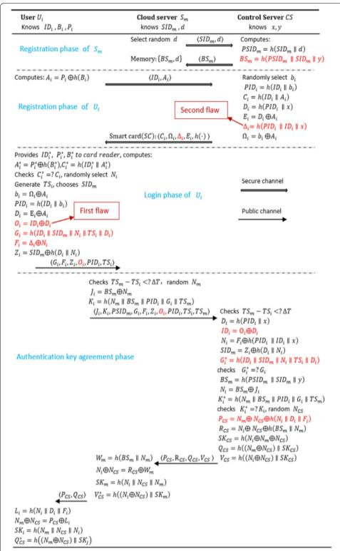
**Fig. 2** Implementation of Kang et al.'s protocol. Implementation of the registration, login, and authentication key agreement phases in Kang et al.'s protocol
