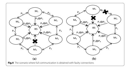
Equation 13 shows that row one is zeroed because  $M_1$  is the dead member; hence, the way to retrieve the all member's data is similar to the case when one wire is disconnected.
