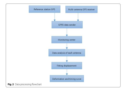
the reference station and the measuring point, and time sequence analysis, the predicted deformation trend curve can be generated, as shown in Fig. 2 [19].
