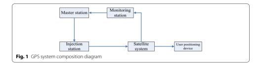
is 1.58 h. Four satellites are deployed on the plane, and the coverage angle is 55 degrees [8, 9]. In actual use, the GPS system receiver can capture more than 4 satellites. At this time, in order to improve the positioning accuracy, the receiver divides the captured satellites into several groups according to the constellation distribution, with 4 satellites in each group. After calculation and analysis, the group with the smallest error is selected for positioning calculation.
